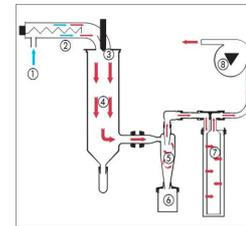
The mini Spray Drier B-191 functions according to the same principle as the co-current flow atomizer, the sprayed product and drying air flow are in the same direction.
